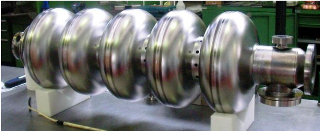
Figure 6: Picture of the full cavity after final welding
