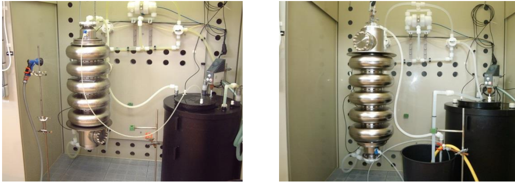
Figure 9: (left) First chemistry process and (right) second one after 180° rotation of the cavity
