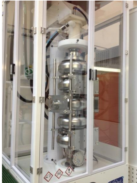
Figure 9: 704 MHz 5-cell cavity installed in the vertical electropolishing set-up
