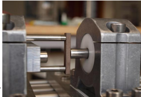
Fig. 14: Maximum bending strength obtained in dynamic conditions, using a new Split Hopkinson Pressure Bar (SHPB) setup, shown on the right. Achieved strain rates are close to 10^4 \text{ s}^{-1} . POLITO
