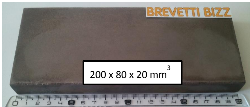
Fig. 4: A large Mo-CD sample produced by liquid infiltration. Brevetti Bizz
