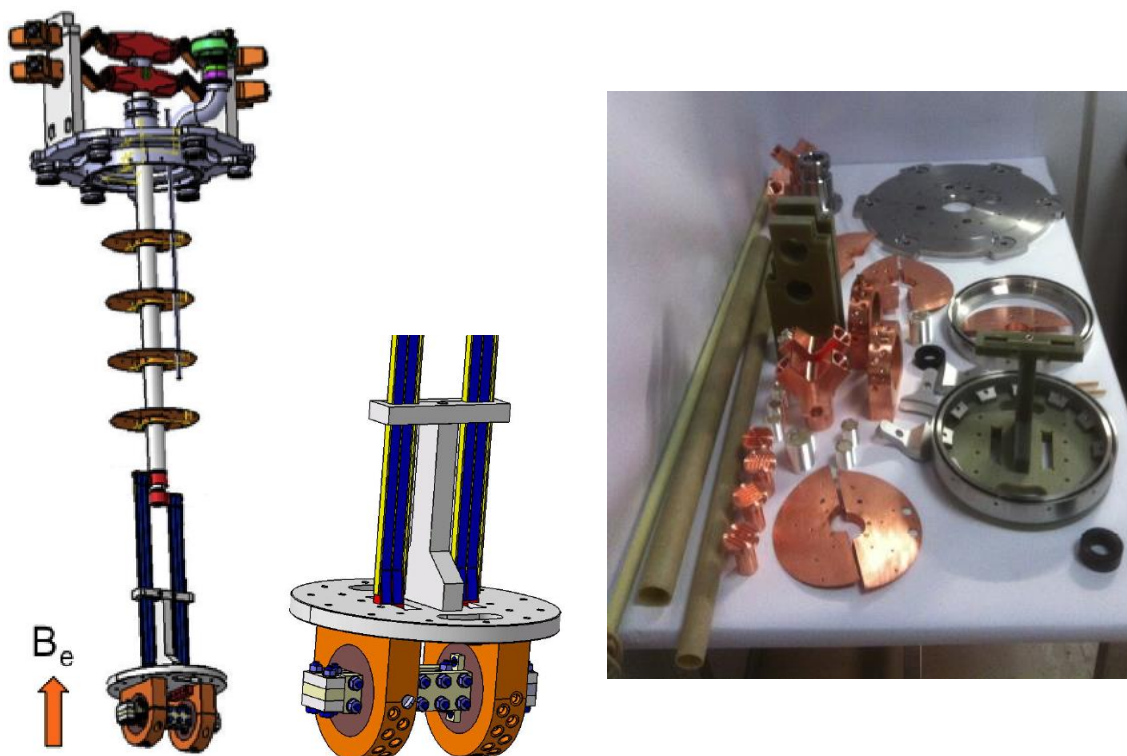
Figure 6: Test set up to study the pancake under different field orientations (left 2 pictures), all the components of the setup (right).
