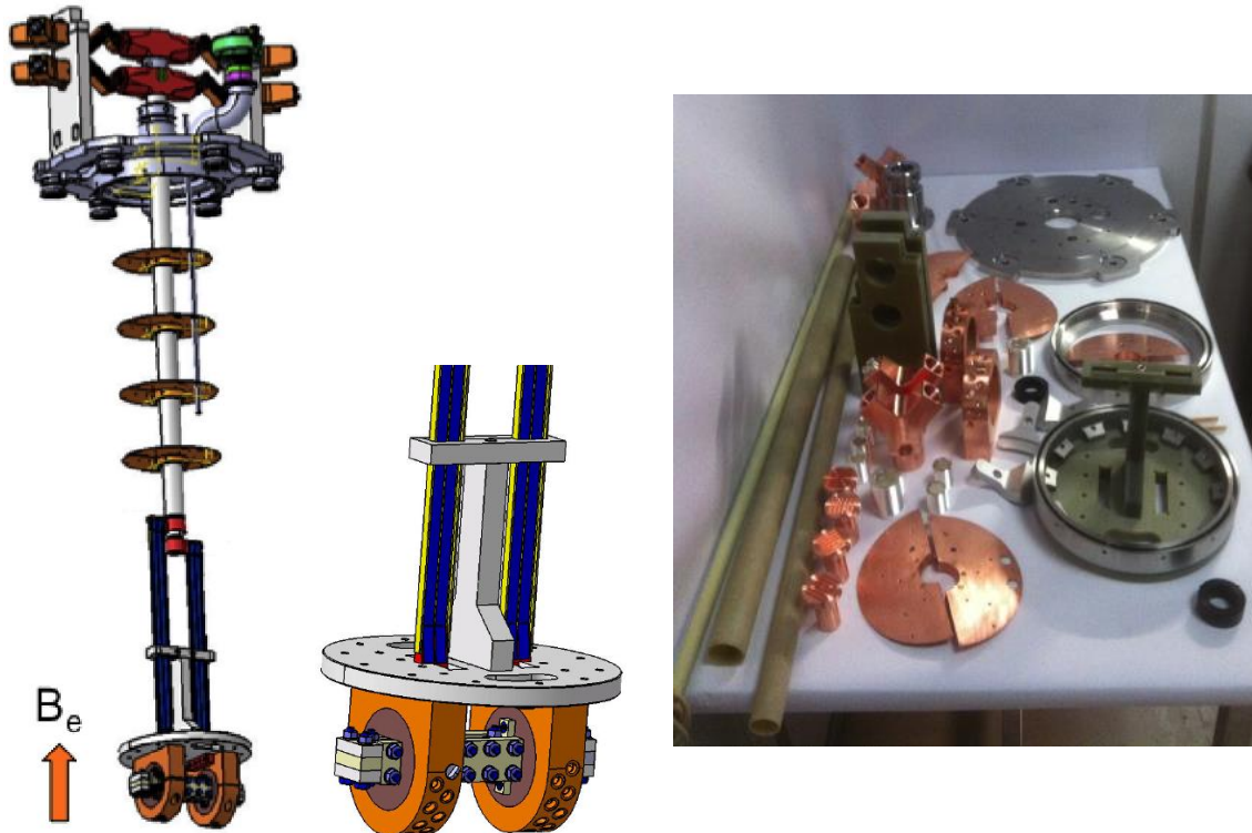
Figure 4: Test set up to study the pancake under different field orientations with all the components.
