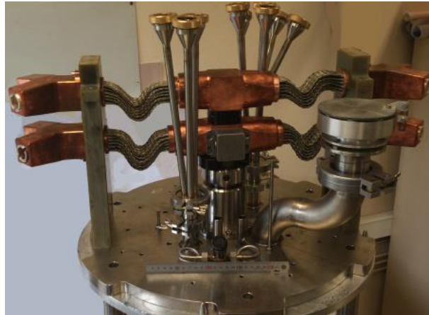
Figure 7: top of the setup with the two 3 kA current leads, some connectors for instrumentation, the two helium transfer tubes and the safety valve.
