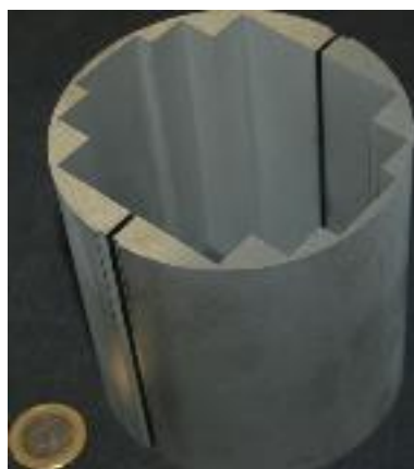
Figure 16: First tests of wire cutting of a pad of 100 mm at LNCMI.
