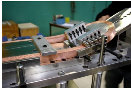
Fig. 9.2.1 – Winding tests with flared end turned up.
