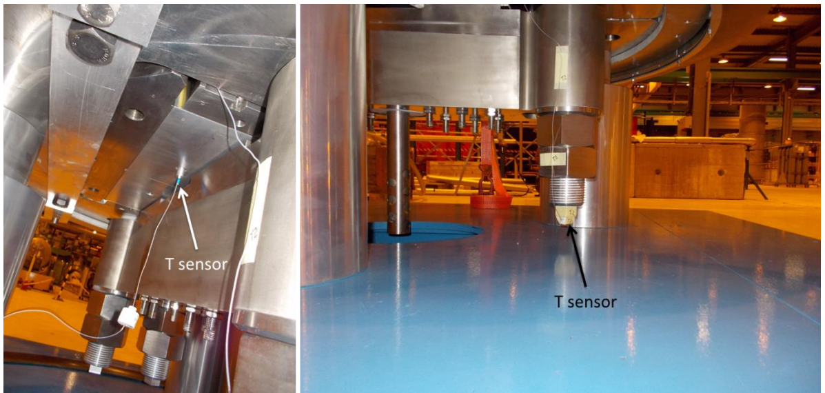
Fig. 9.8.6 – Temperature sensors at the bottom of the magnet structure: dummy and rod.
