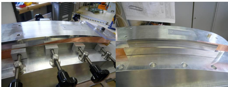
Fig. 9.3.1 – Layer jump test with one chicane (left) or two chicanes (right).
