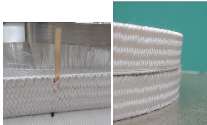
Figure 11: details of the coil, a) voltage tap, b) alignment of the 2 layers in one end.
