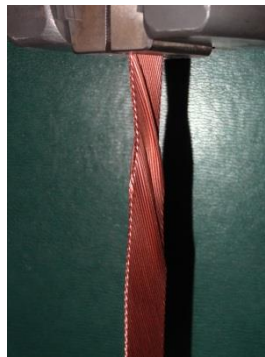
Fig. 9.5.3 – Traction test on FRESCA2 cable.
