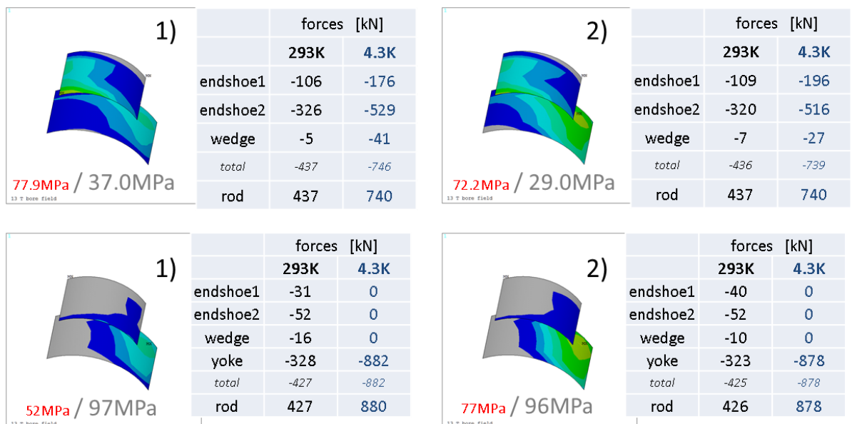
Fig. 7.1.20 – Compression stresses on the coil/post contact (ends), with non-impregnated wedge. Pre-load on the end-shoe + wedge (top) or on the end-shoe + wedge + yoke (bottom) 1) with 2) without lateral wedge/pad contact.
