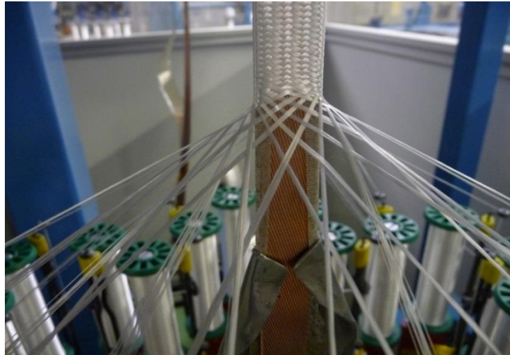
Fig. 5.3.1 – S-grade fibre-glass braided around a cable.
