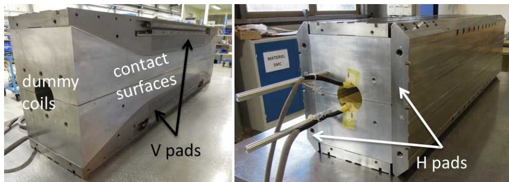
Fig. 8.4.10 – Coil-pack with dummy-coils.
