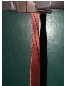
Fig. 9.5.3 – Traction test on FRESCA2 cable.
