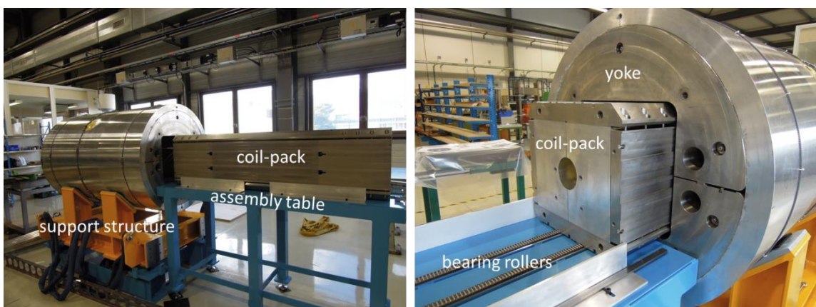
Fig. 8.4.21 – Assembly table, insertion of the coil-pack.
