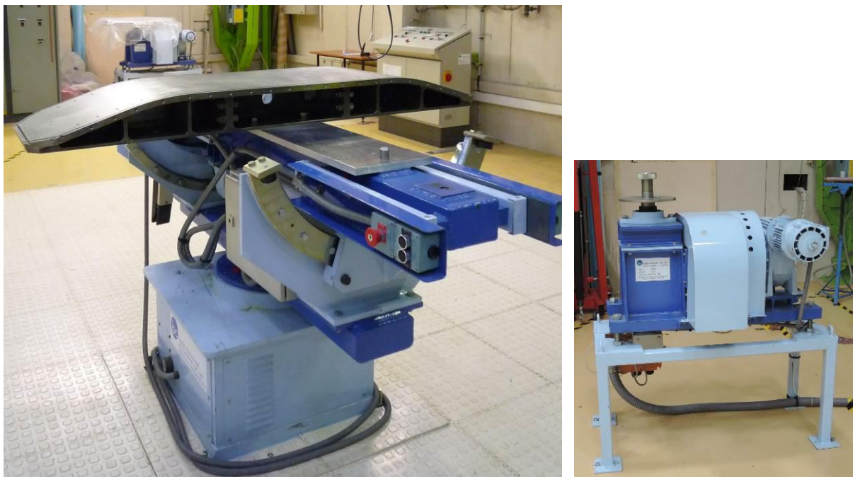
Figure 2: a) winding table installed on the winding machine b) electromagnetic brake.
