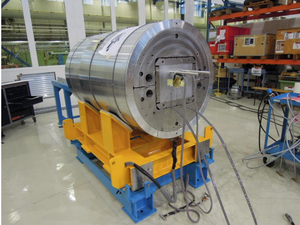
Fig. 8.4.22 – Coil-pack inserted into the yoke.
