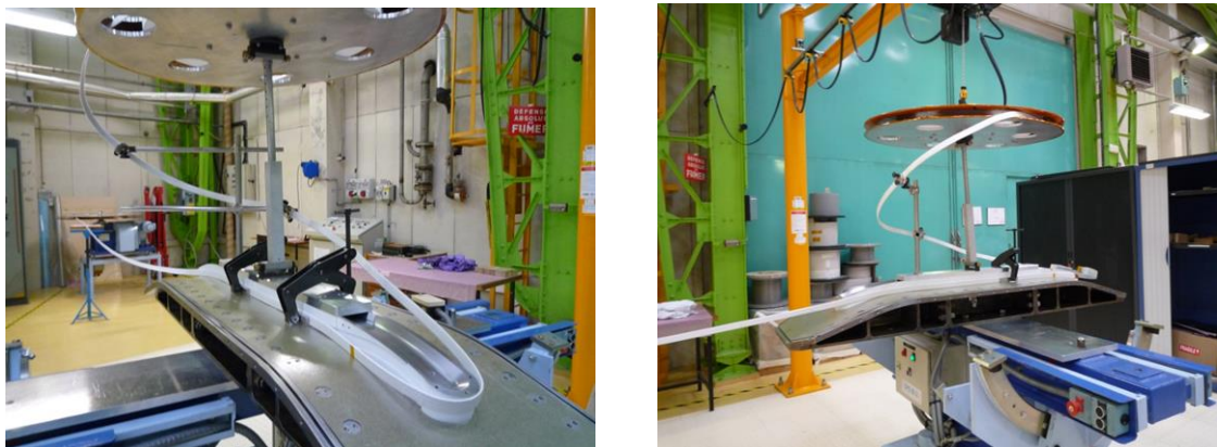
Figure 4: the two coils in position for the winding of the first layer.
