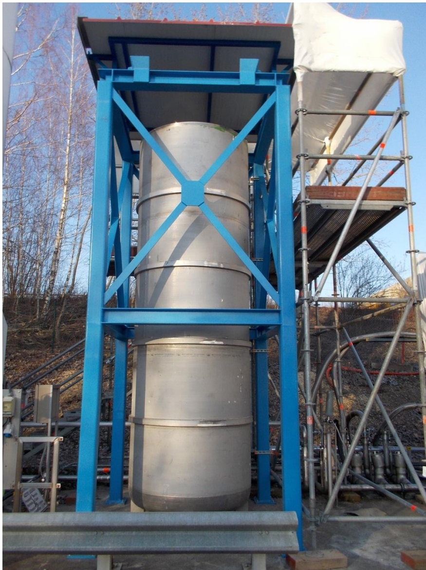
Fig. 9.8.9 – Vessel of \varnothing 1.2\text{m} \times 4\text{m} for the cool-down test outside of SM18.
