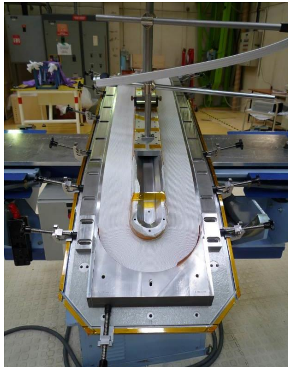
Figure 8: winding of the coil: test of horseshoes + rails closing on the layer 4.
