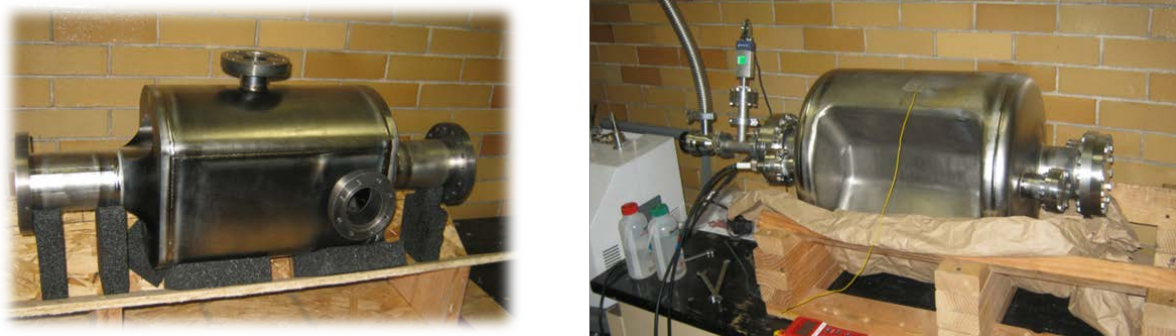
Figure 10: Prototype compact Nb-Ti crab cavities for the LHC: 4-rod cavity (left) and double-ridge cavity (right).
