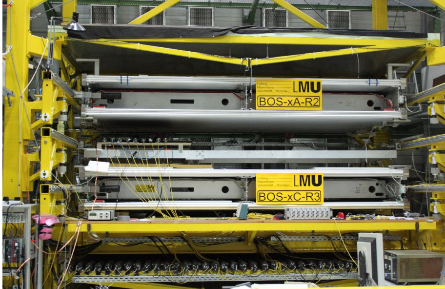
Figure 11. The Munich University Cosmic Ray Facility, with two 9m 2 BOS MDT chambers for cosmic muon reference tracking, together with a prototype micromegas chamber in between, being read out by the SRS based Micromegas ROD.
