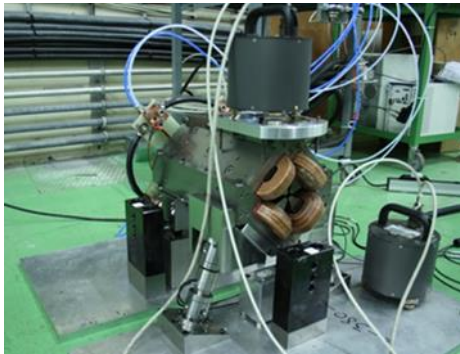
Figure 34: Left: Powered quadrupole with water cooling
