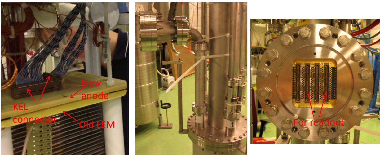
FIG. 81: Prototype of the signal feedthrough flange with 4 connectors.
