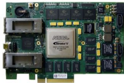
FIG. 74: FPGA processing board based on Stratix V from Altera. The board features a dual QSFP+ cages for 40GigE or 10GigE links, 16 GBytes DDR3 SDRAM, 72 MBytes QDR II/II+, two SATA connectors and is programmable via OpenCL.
