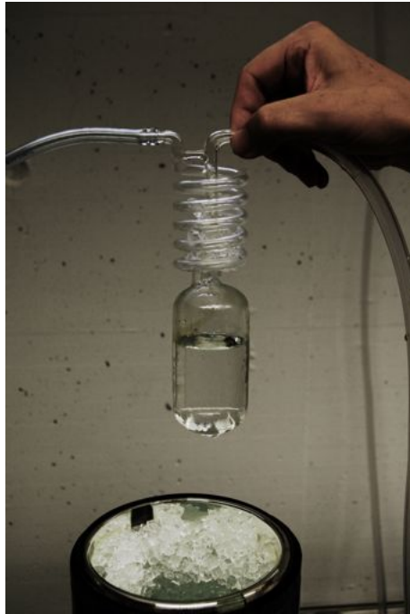
FIG. 103: Collected water from regeneration of a copper cartridge.
