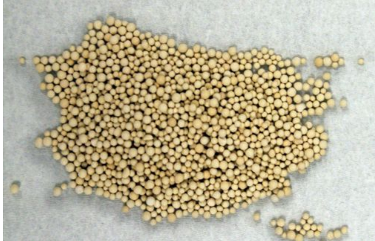
FIG. 101: Molecular sieve ZEOCHEM 3A ® grains before inserting them in the regeneration cartridge. Each grain has a diameter of about 2 mm.
