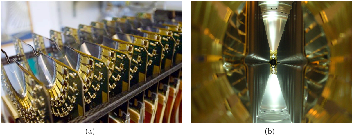
Figure 2.16: a) VELO modules. b) Interior of the RF foil, viewed in the open position.
