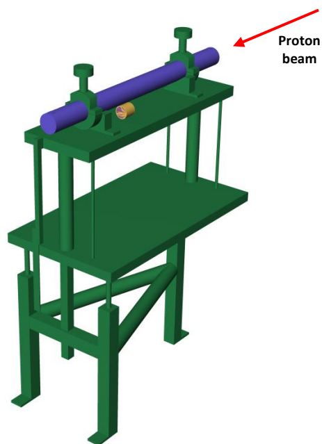
Figure 5.13: Detail of the irradiation set-up used in the FLUKA geometry. The aluminium target holder is shown in green, the copper target in blue and the irradiated soil sample in brown. The drawing is obtained using SimpleGeo [35].
