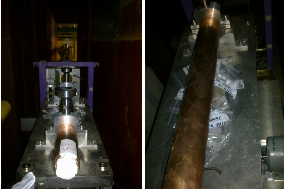
Figure 5.12: H4IRRAD target area. The samples were installed on the aluminum table just below the copper target.
