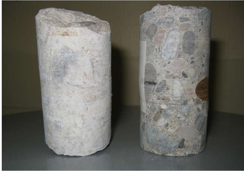
Figure 4.4: Comparison between "heavy" barytes concrete (left) and "light" concrete samples (right).
