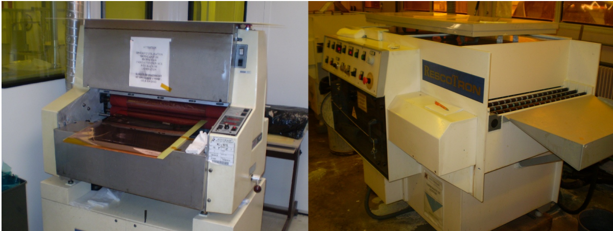
Figure 2.5: Photoresist laminator and developer.
