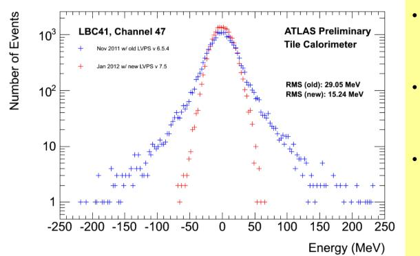
Electronic noise in TileCal is not Gaussian. We approximated it with two Gaussians. Mainly, it comes from the Low Voltage Power Supply (LVPS) providing power for front-end electronic.
