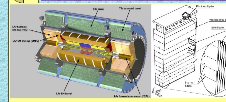
**Overview of the Tile Calorimeter of the ATLAS detector** Total length is 12 m, diameter - 8.5 m
