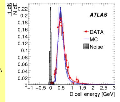
• The truncated mean of the dE/dx for cosmic and testbeam muons shown per radial compartment and, at the bottom, compared to Monte Carlo. • For the cosmic muon data, the results were obtained for modules at the bottom part of
