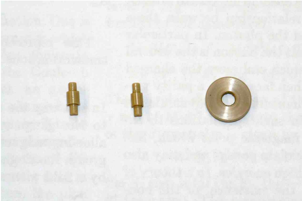
Figure 2.70.: Picture of both types of pintles, 2.80 mm (left), 2.60 mm (center) and the washer (right). The pintles and the washer are made of Peek.
