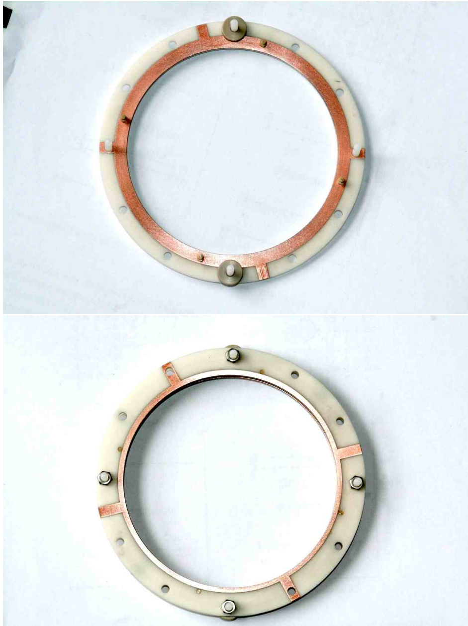
Figure 2.71.: The bottom ceramic ring equipped with the pintles and the washers (top). The ceramic stack equipped with the pintles and the washers (bottom).
