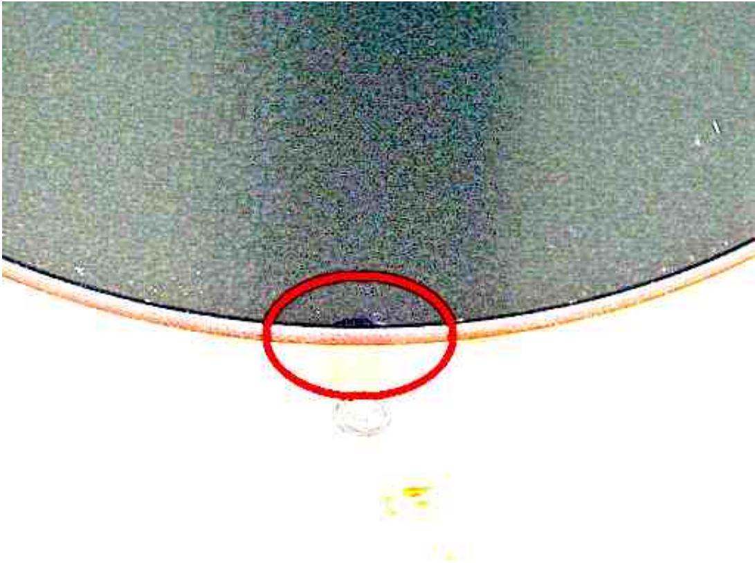
Figure 2.6.: The mark of the front microchannel plate is highlighted with the red circle.
