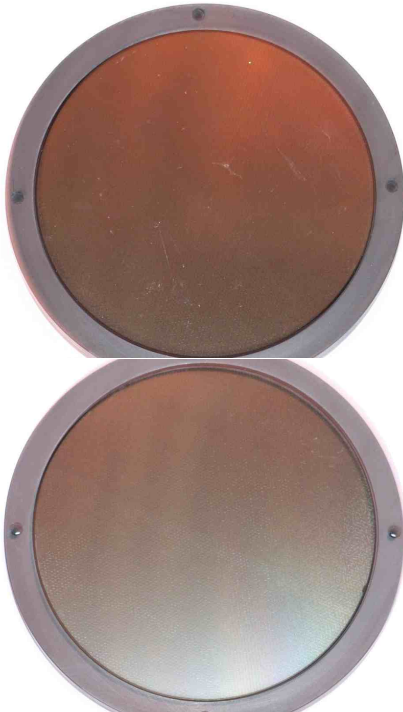
Figure 2.7.: Pictures of the front MCP laying in the transport box from the front side (top) and the back side (bottom). The top side of the MCP has been longer exposed to atmosphere, why it is more contaminated with dust.
