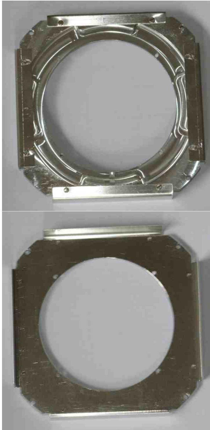
Figure 2.15.: Pictures of the mounting plate placed from the top and back side. On each of the four sides L-shaped metal plates are installed to protect the delay line anode from the sides. Two of them can be slid to side to bear the notch with can hold the ceramic ring of the back MCP. By sliding back the L-shaped plate and attaching it with each two screws the ceramic ring becomes attached to the mounting plate.
