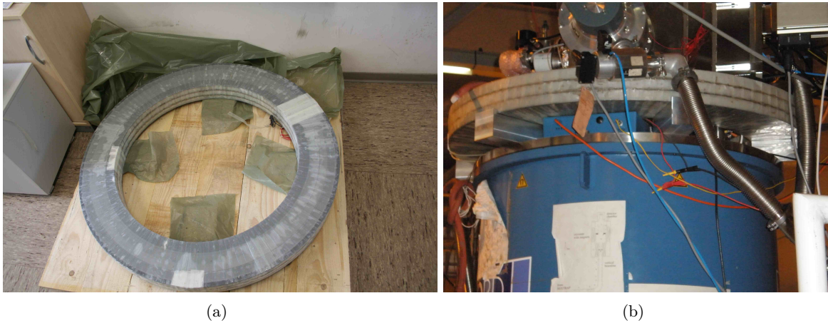
Figure 3.7.: Pictures of the compensation magnet just unpacked right after delivery from the company (a). The compensation magnet after installation on top of the cryostat, holding the two superconducting magnets (b).
