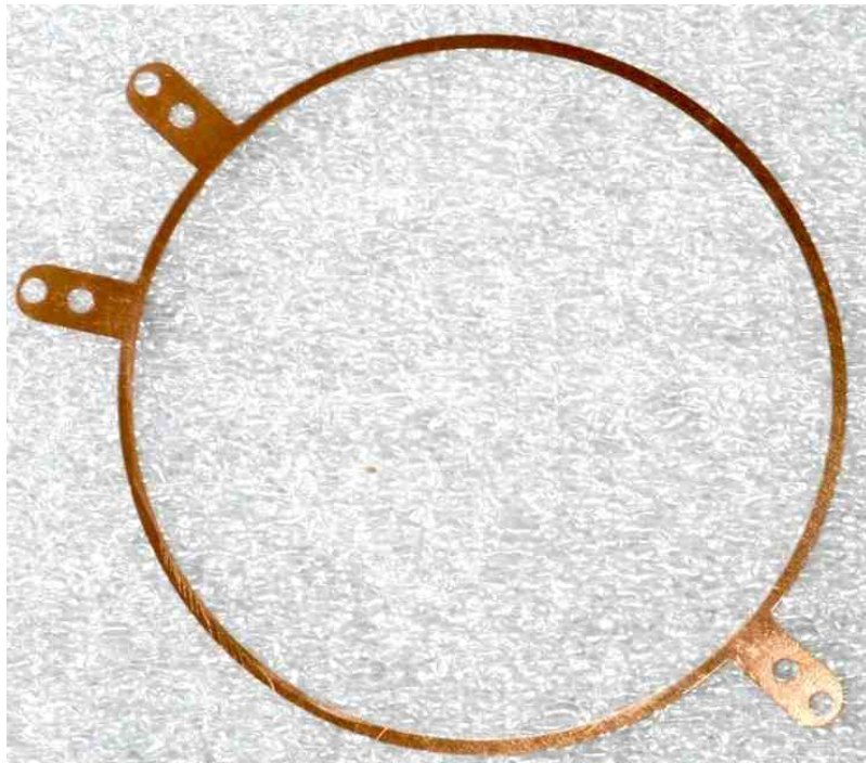
Figure 2.66.: Picture of one of the shim rings from Roentdek with three lugs to support the ring and connect an electrical contact.
