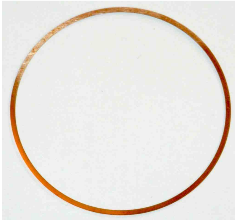
Figure 2.67.: Picture of the shim ring manufactured in the mechanical workshop in Münster, which is placed between the MCPs. This ring was manufactured from a sheet of CuSn8 bronze by the use of wire-electro discharge machining.
