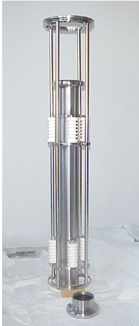
Figure 5.11: Picture of the pulsed drift section with Macor insulators and its support structure.
