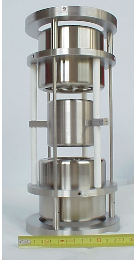
Figure 5.8: Electrode structure of the einzel lens of the horizontal beamline.
