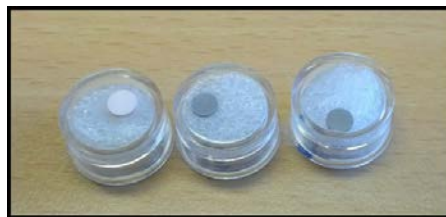
Figure 3. Pellets of ^{146}\text{Nd} , ^{170}\text{Er} and ^{203}\text{Tl} before their irradiation at ILL.
