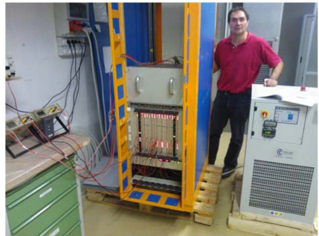
Fig. 7. The setup used for the test. To the left there are the voltmeters reading the PS currents and the T sensors, in the center the rack with, from the bottom, the fan tray, the bin filled in with the load boards, the heat exchanger and the PS, and to the right the chiller.
