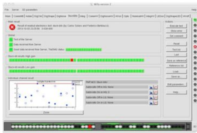
Fig. 6. The stuck bit test is a new functionality test which detects upset bits that can cause failures in the digitizing process.
