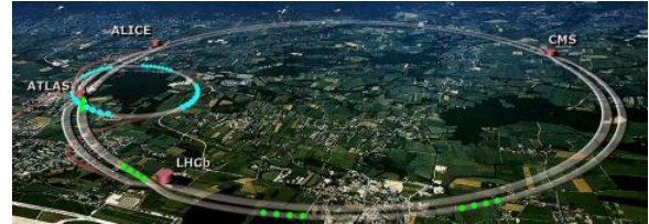
Fig. 1. The LHC lies beneath the French-Swiss border. Its circumference is 27 km and its designed collision energy is up to \sqrt{s} = 14 \text{ TeV}
