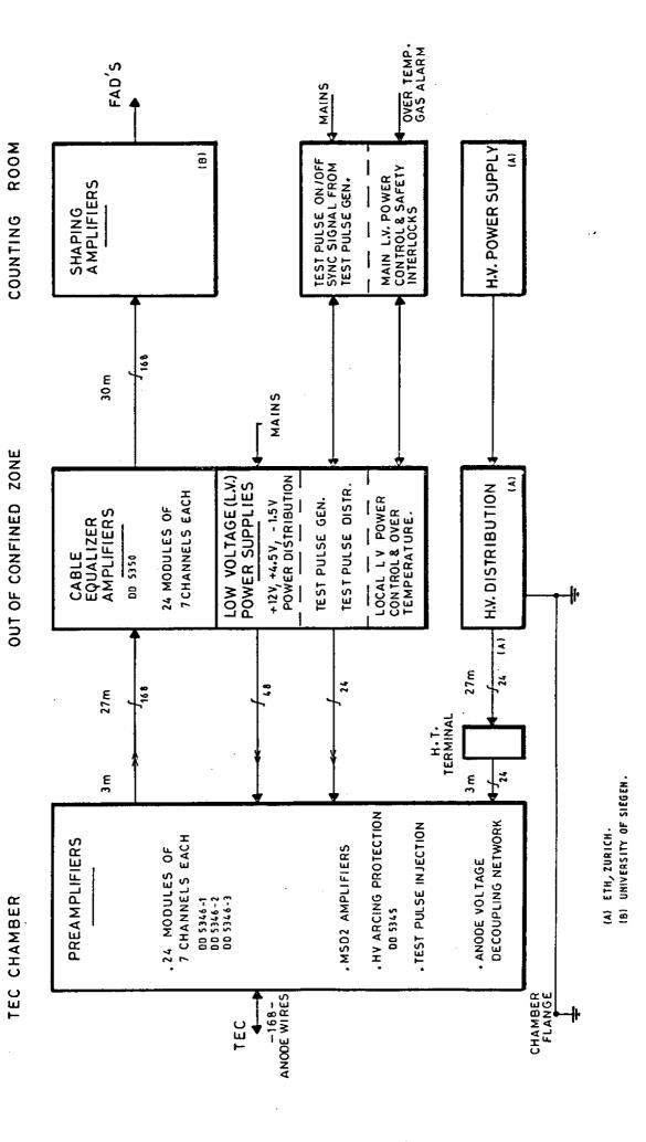
Fig.1 — Block Diagram of the TEC MARK-J Analog Readout.
