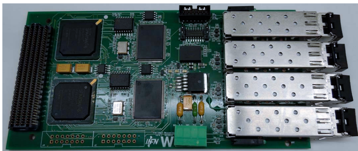
Figure 2. The left picture shows a prototype of the current FTK_IM card with a “FPGA Mezzanine Connector” element, two FPGAs, and S-link connectors. The right figure shows the clustering scheme with a small grid size, 5 \times 5 . The search region is the orange box, which is aligned so that the first incoming hit is placed at the middle of the left side. Data from the same columns, shown in the blue box, are temporarily stored in a separate RAM. After a cluster is read out, the grid is realigned to the next left-most hit.
