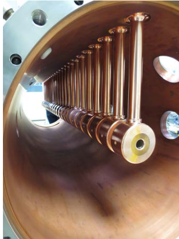
Figure 18: First segment of Linac4 DTL with drift tubes.
