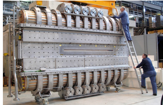
Figure 10: PSI 50 MHz normal conducting cavity [2]
