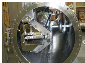
Transversal side view of the electrostatic septum magnet
