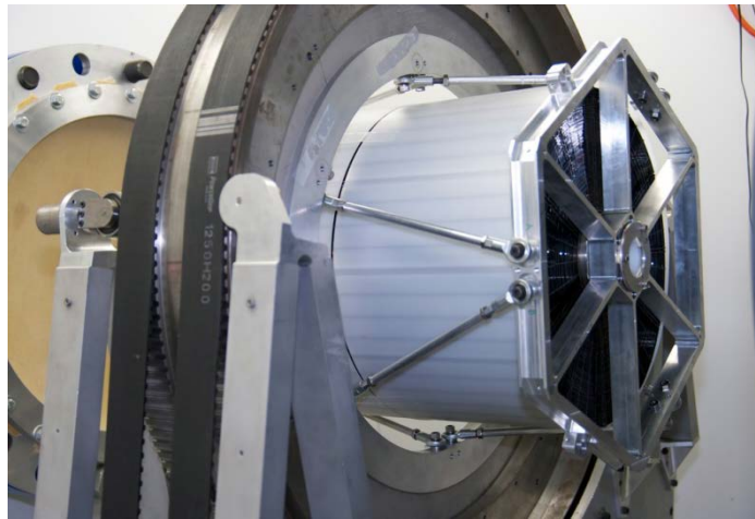
Figure 47 - NuSTAR X-ray telescope during on-ground calibrations at Columbia University. The optic, which is a conical approximation to a Wolter-I telescope, consists of 6 sectors. The supporting spider structure can be seen in the right part of the image. For CAST, only one sector of a NuSTAR-like optic needs to be built.
