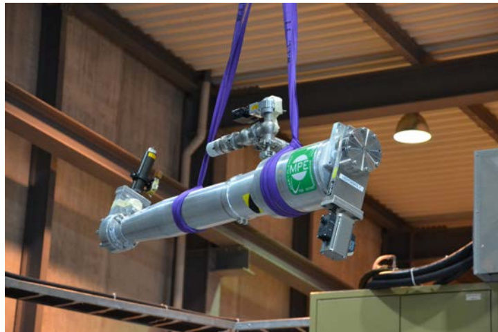
Figure 19 - MPE X-ray telescope being removed from the CAST beam-line.
