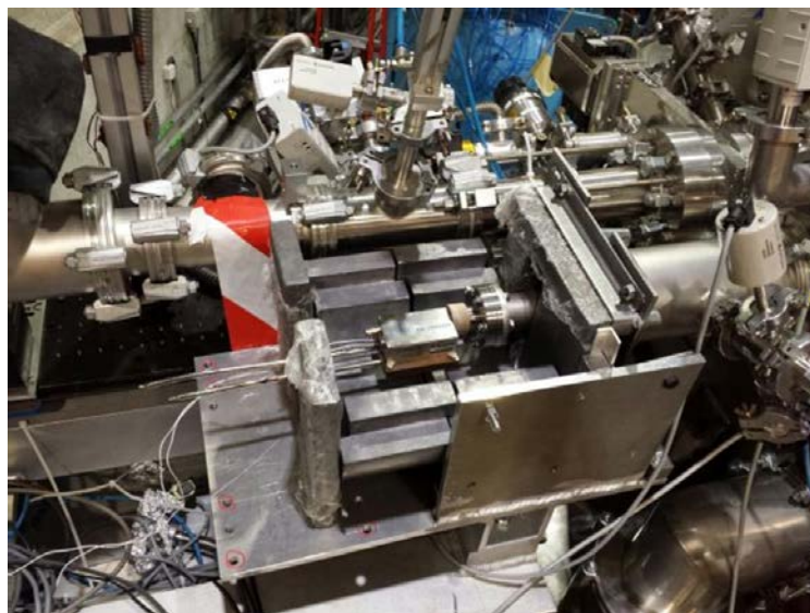
Figure 25 - The SDD installed in CAST together with half the shielding.
