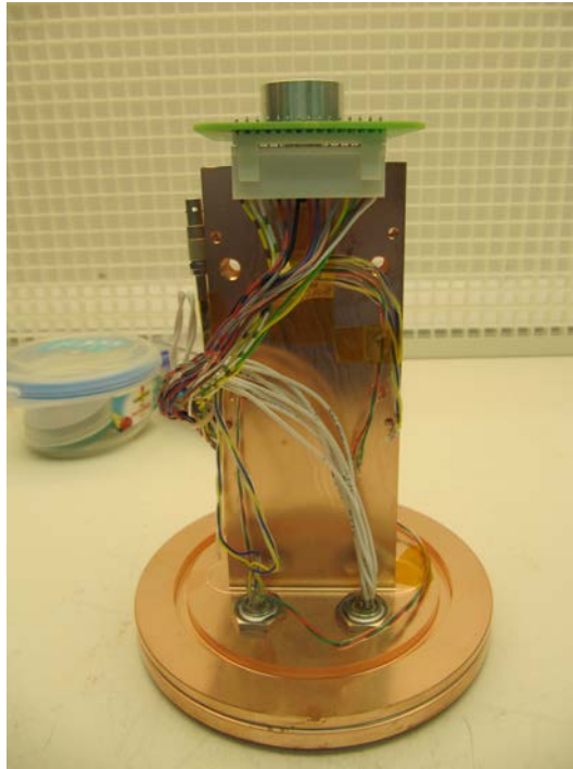
Figure 29 - Large SDD mounted on copper plate, which acts also as the preamp holder and heat sink for the detector.
