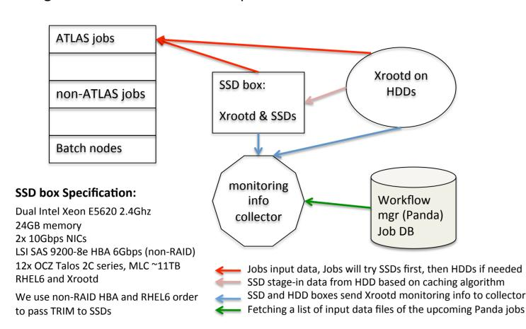
Both SSD and HDD storage systems run Xrootd. ATLAS jobs will read SSDs first, and will read from HDDs if and only if data is not available on SSDs
