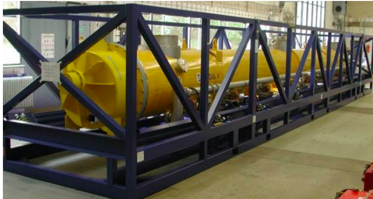
Figure 3.23 An European XFEL prototype cryomodule in its transport frame. The module is supported on vibration dampers [46]
