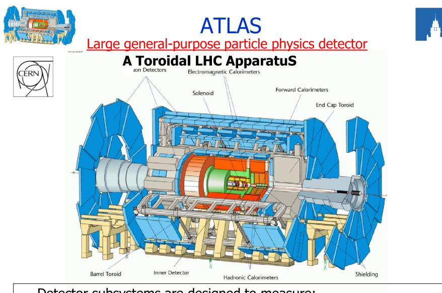
Detector subsystems are designed to measure: energy and momentum of  $\gamma$  ,e,  $\mu$ , jets, missing E<sub>T</sub> up to a few TeV
