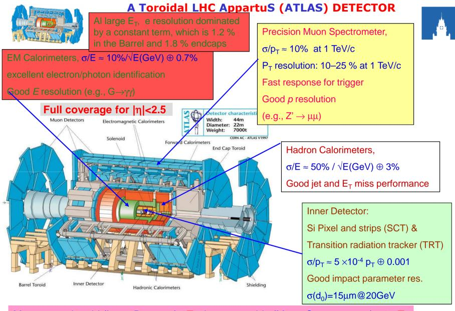
Magnets: solenoid (Inner Detector) 2T, air-core toroids (Muon Spectrometer) ~0.5T
