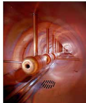
Figure 2.2: Drift Tubes in the LINAC facility at Fermilab 2
