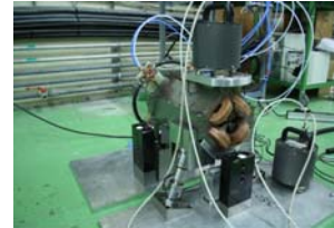
A CLIC Main Beam Quad prototype on two stabilisation actuators. Image credit: CERN
