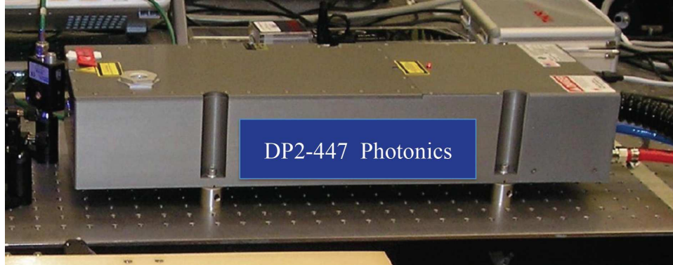
Figure 4.3: Laser monitoring light source, diode pumped \text{YVO}_4 laser 1 by Photonics.
