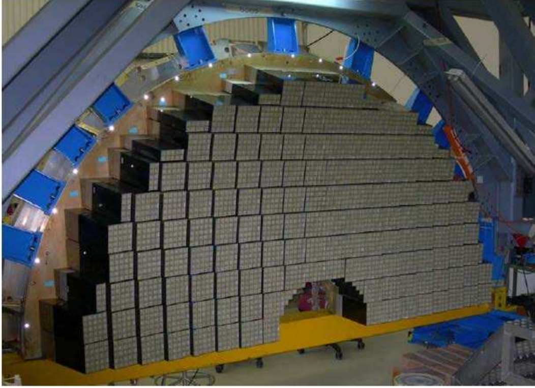
Figure 3.14: The CMS Electromagnetic calorimeter, endcap Dee.
