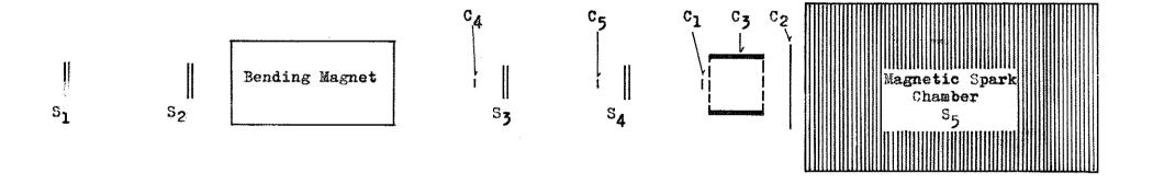
FIG. 1: Diagram of apparatus: Trigger on  $C_4C_5C_1C_2C_3$  with constraints on acceptable pulse heights in C1 and C2.
