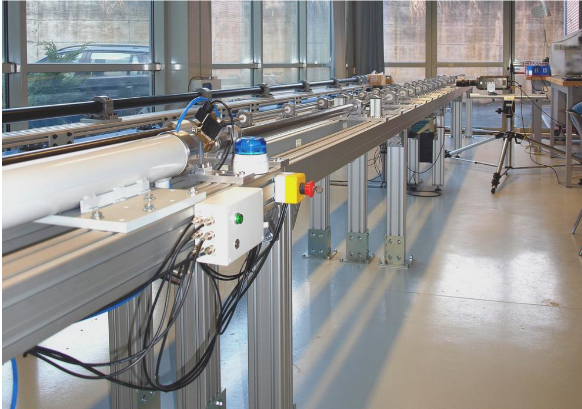
Figure 6. SHPB setup used for high dynamic tests of the Mo-CD samples.
