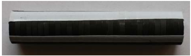
Figure 6: Stack of the graphite discs irradiated with Tantalum ions.
