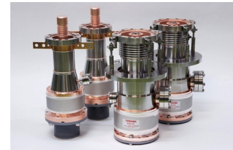
(b) Two sets of completed STF-2 input couplers
