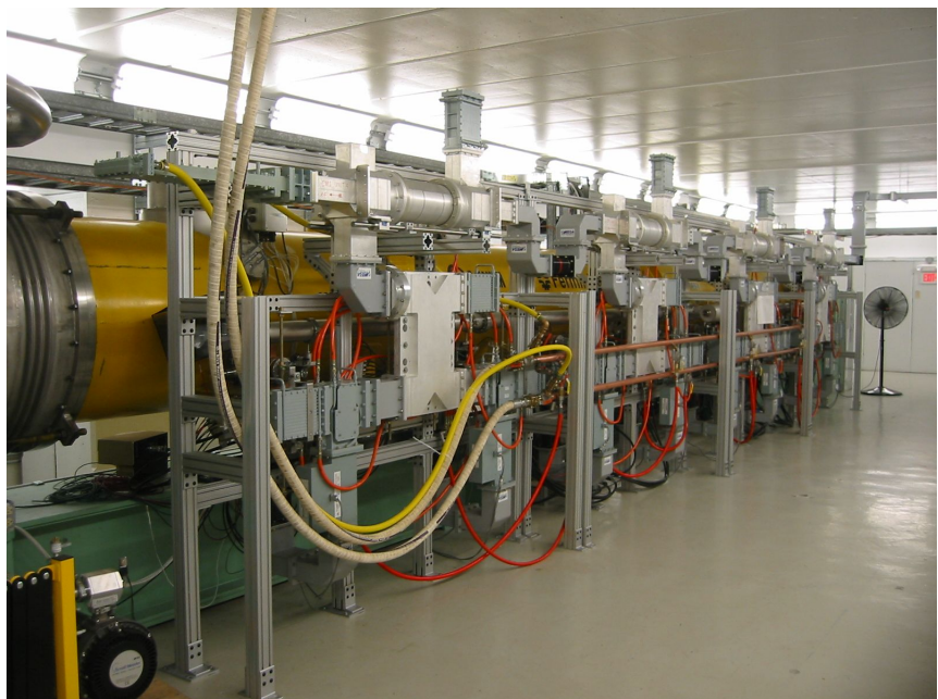
Figure 3.27 Cryomodule 1 installed for operation at Fermilab's NML building. The waveguide distribution system, which feeds RF power to all 8 cavities simultaneously, is in the foreground.
