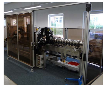
(b) The tool for field-flatness tuning and geometric adjustment of 9-cell cavities.
