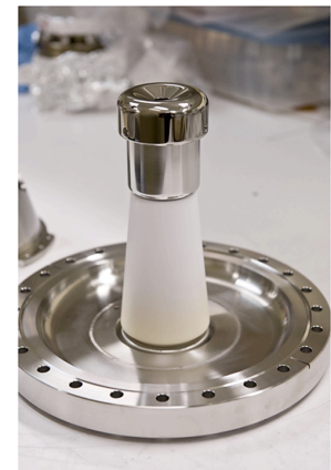
Figure 4.5 Compact inverted insulator with test electrode used to evaluate electrode materials, polishing techniques and inert gas processing.
