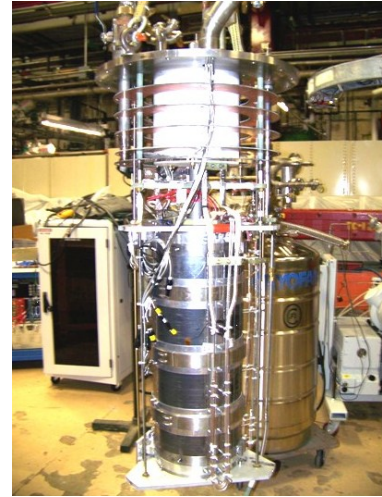
(b) The split quadrupole mounted on the insert of the cryostat.
