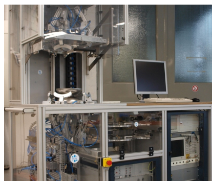
(a) HaZeMeMa, the tool for room-temperature RF measurement of half cells
