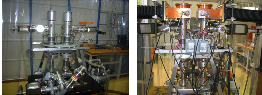
(a) Two couplers being conditioned
