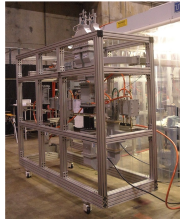
(b) A two-feed unit of PDS2, incorporating a VPD, ready for high-power testing at SLAC.
