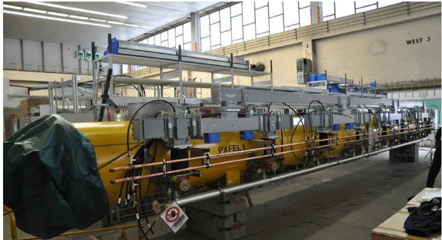
Figure 2.55 European XFEL-type waveguide distribution tested on the cryomodule ACC7 at FLASH.
