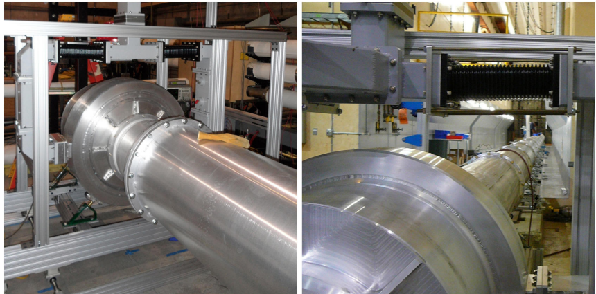
Figure 2.71 Views of a CTO used as a launcher or coupler in high-power tests of KCS WC1890 main waveguide runs.
