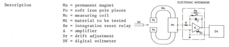
The set-up is original in that a small permanent magnet is used to produce the required field level. When a piece of material of magnetic susceptibility  $\kappa << 1$  is brought into the gap, the magnetic flux in the coil varies by a small amount proportional to  $\kappa(1-\kappa)$ . The signal induced into the coil is fed via an electronic integrator to a digital voltmeter calibrated directly in values of  $\kappa(1-\kappa)$ .
