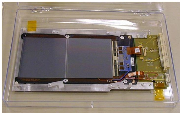
Figure 2.2: The CMS silicon microstrip detector; two silicon sensors of about 10 \times 10 \text{ cm}^2 , the support frame and the frontend electronics are visible [44].
