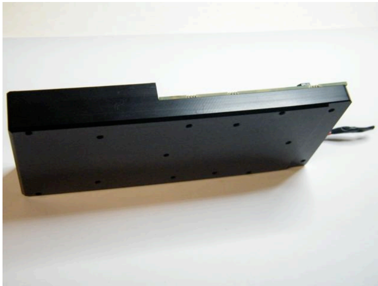
Figure 5.4: The MARS chip carrier enclosure is made of acetal, dyed black for light tightness
