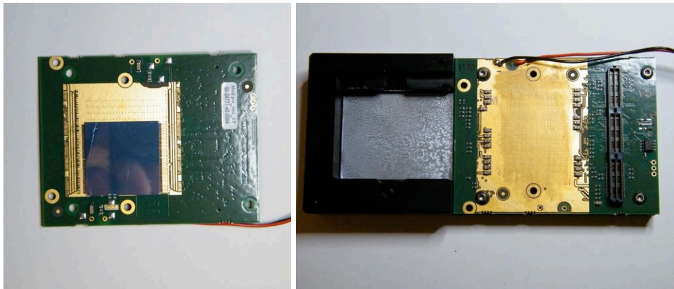
Figure 5.3: Left Hex silicon Medipix3 chip carrier with quad silicon Medipix3 fitted as seen when sensor side unprotected by acetal block. Right The same chip carrier seen from the back side, fitted into the protective block. The metal heatsink deep in the block has a patina of conductive thermal grease. When installed in a camera, this surface is in contact with the underside of the Peltier heatsink plate. The 180 pin Samtec plug is visible on the right of the printed circuit board.
