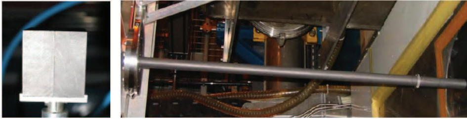
Figure 3.7: Pictures of the thin (left) and T2K replica (right) targets, which are used for the NA61 data taking for T2K.
