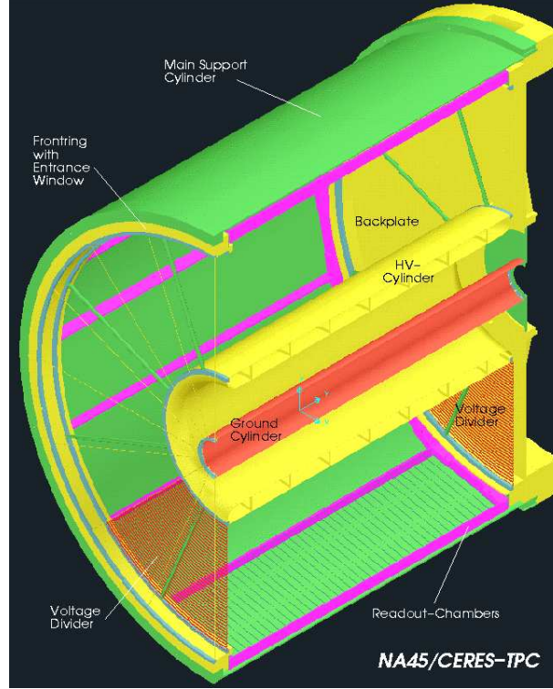
Figure 2.8: General view of the TPC.
