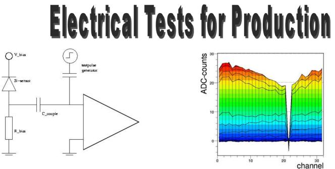
Pinholes less easy to detect - but Beetle seems to be stable at high leakage Operating at -0.5 Volts bias affects response (currents, working point)
