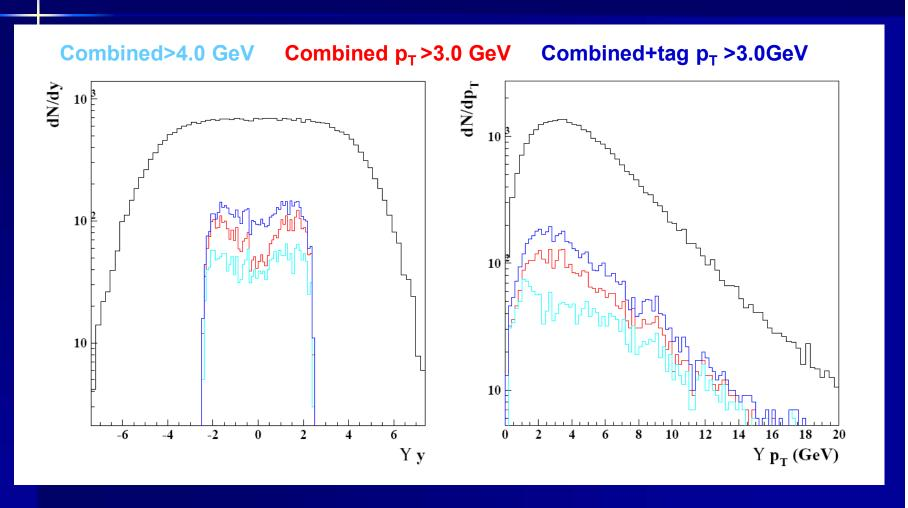
Muons from Y decays are more energetic and they can be reconstructed over a large Y kinematic range
