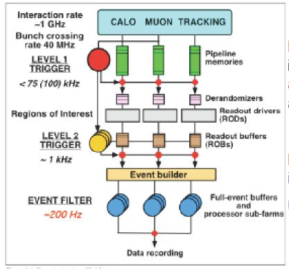
LVL 1 di-μ trigger can be based on φ information from μ-trigger chambers for a low p<sub>T</sub> cut (toroidal B bending is in η), and defines Regions of Interest.
