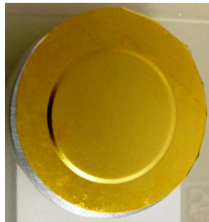
Figure 4: A photograph of one of the gold foils, mounted in the holder. The foil is glued to the edges and subsequently the central part of the holder is tightened against it such that the central part protrudes and is kept flat.
