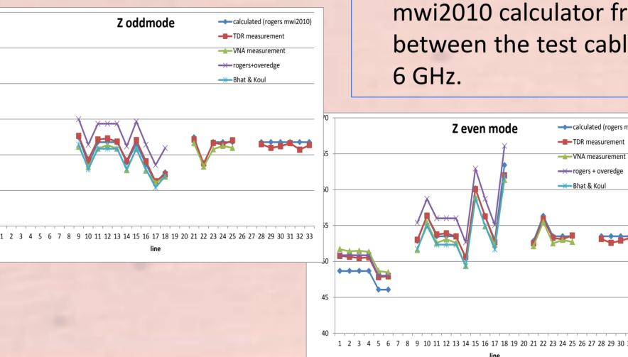
Comparison between impedance at measurement and calculation. (Odd and Even mode)
