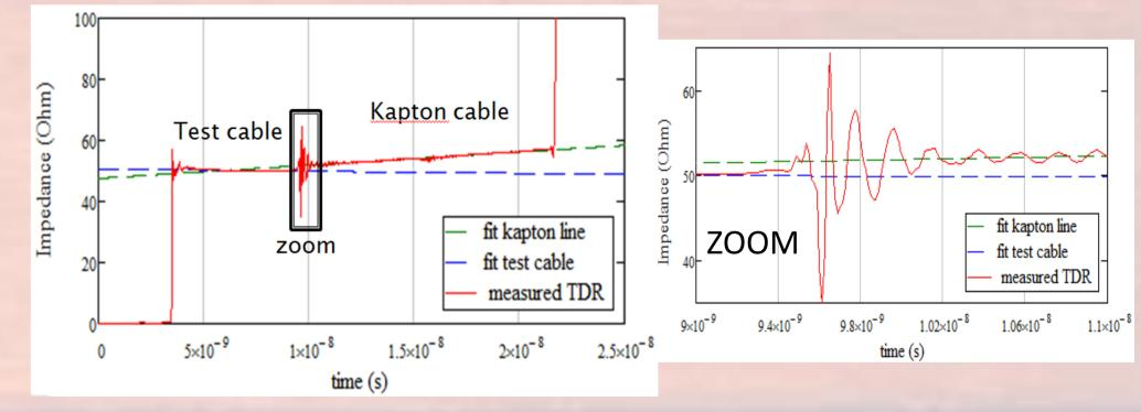
Impedance measurement along the test and measurement (Kapton) cables.
