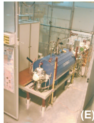
Figure 3.7: (A) The Trap-EBIS combination. (B) Sketch of the bunching process in the Penning Trap : cooling of the incoming RIB is done through collisions with the buffer gas. (C) Sketch of charge breeding process in the EBIS : after bunching in the Penning Trap, the ions are re-accelerated to 20-60 kV and confined within potential barriers in the EBIS. (D) Picture of the Penning Trap. (E) Picture of the EBIS, the cylinder contains the liquid He for cooling of the superconducting magnet. Pictures taken from [ISO06].
