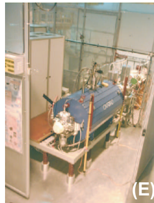
Figure 3.7: (A) The Trap-EBIS combination. (B) Sketch of the bunching process in the Penning Trap : cooling of the incoming RIB is done through collisions with the buffer gas. (C) Sketch of charge breeding process in the EBIS : after bunching in the Penning Trap, the ions are re-accelerated to 20-60 kV and confined within potential barriers in the EBIS. (D) Picture of the Penning Trap. (E) Picture of the EBIS, the cylinder contains the liquid He for cooling of the superconducting magnet. Pictures taken from [ISO06].
