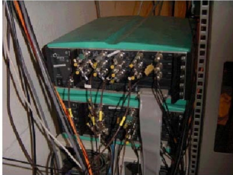
Figure 3.15: The Acqiris digitisers and the chassis;
