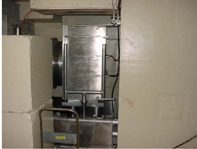
Figure 2.4: The Pb spallation target. It is possible to note on the left the TOF tube and on the right the cooling system.
