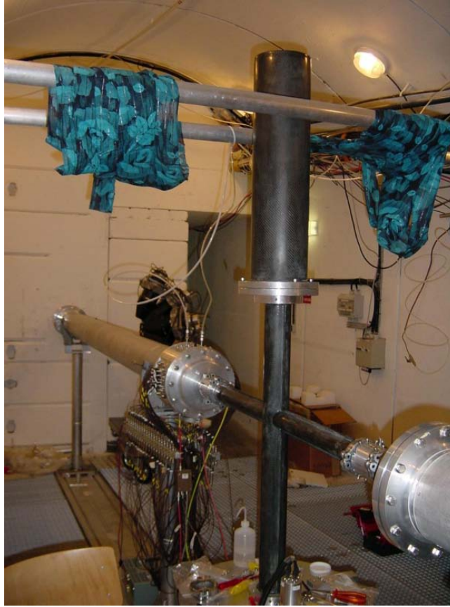
Figure 3.8: Carbon fibre Sample changer for the measurements of the sample in the vacuum.
