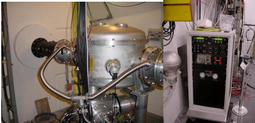
Figure 3.13: The vacuum chamber of the PPAC detectors (left) and the associated gas and safety control unity (right).
