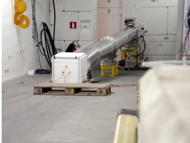
Figure 2.7: Neutron Escape Lane area. At the end of TOF tube is evident the polyethylene block for the beam dump.
