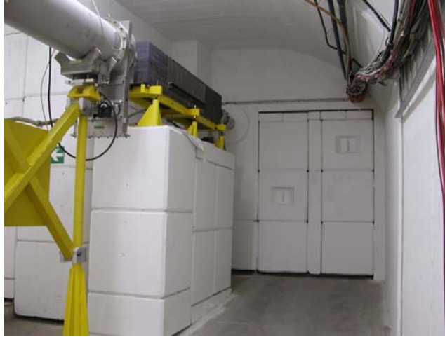
Figure 2.6: The second collimator is necessary for the flux reduction in capture measurements.
