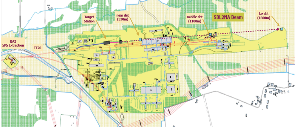
Figure 1: The new SPS North Area neutrino beam layout. Main parameters are: primary beam: 100 GeV; fast extracted from SPS; target station next to TCC2, \sim 11 m underground; decay pipe: 100 m, 3 m diameter; beam dump : 15 m of Fe with graphite core, followed by muon stations; neutrino beam angle: pointing upwards; at \sim 3 m in the far detector \sim 5 mrad slope.
