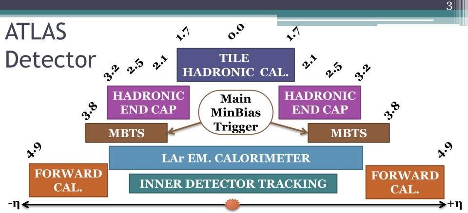
Following analyses use a combination of Inner Detector Tracking and ATLAS calorimetry.
