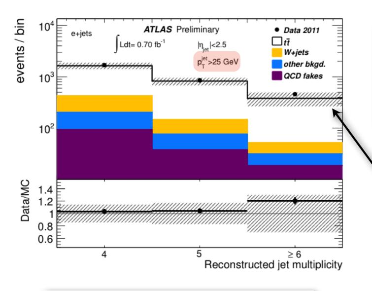
Require one electron or muon and four jets with p<sub>T</sub>>25 GeV
